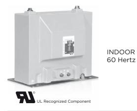
ARTECHE UC/UX/VC series are dry type indoor service voltage transformers. The core is encapsulated with Type B epoxy resin which provides excellent internal dielectric properties and mechanical strength, ensuring a long mechanical and electrical life. The transformer is maintenance free.
