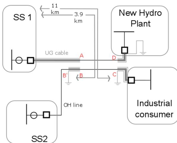
The resulting system would have 3 short underground cable sections that were grounded in just one end, the newest one (the entry to the new hydroelectric plant) being the only one whose earth-connection was conveniently located within the local substation premises thus easing the implementation of a traditional 50G ground overcurrent protection for that cable.
