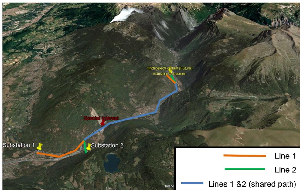
Additionally, there was an overhead line segment crossing a special interest landscape (a riverside landslide of high geologic interest) where the presence of the HV lines was causing a significant visual impact. In order to reduce this impact, RTE decided to underground a segment of both lines which run in parallel in this area.
