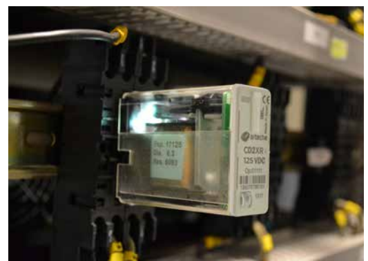
› Heavy duty trip relay during endurance test
