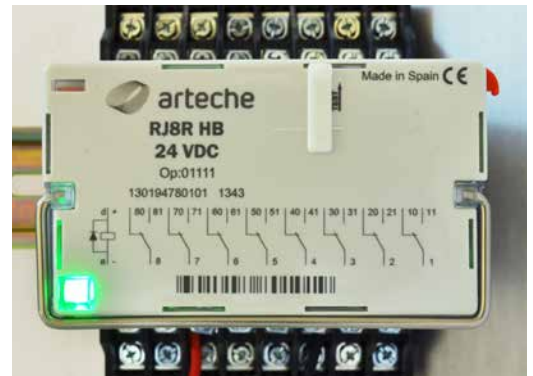
› A self reset tripping relay during operation
