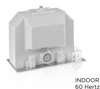
ARTECHE UC/UX/VC series are dry type indoor service voltage transformers. The core is encapsulated with Type B epoxy resin which provides excellent internal dielectric properties and mechanical strength, ensuring a long mechanical and electrical life. The transformer is maintenance free.
