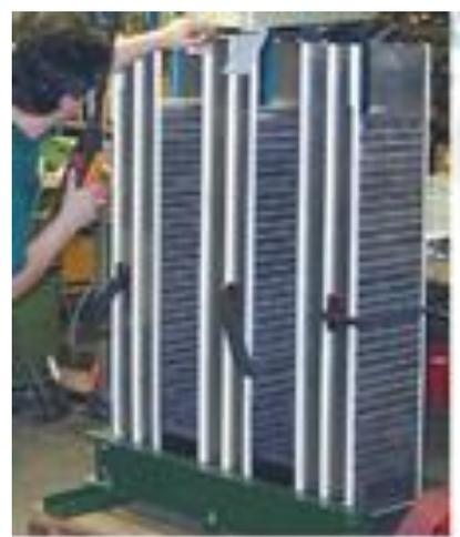
*Partially assembled reactor with PolyGap™ core*
