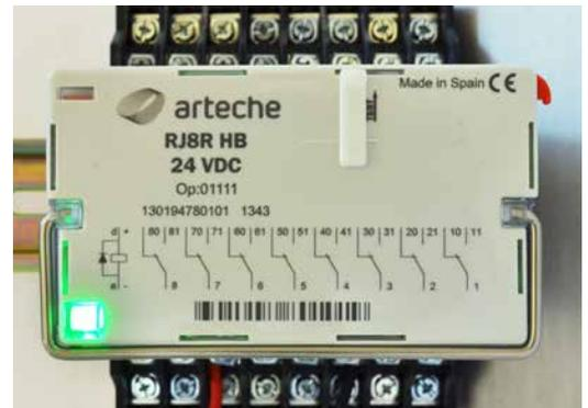
› A self reset tripping relay during operation
