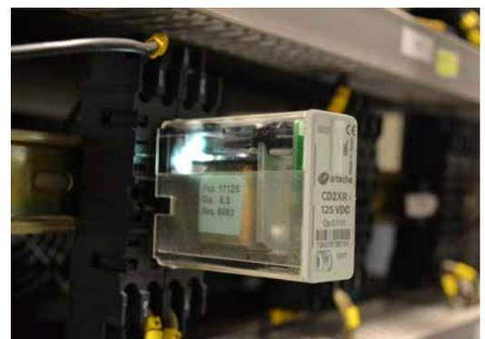
› Heavy duty trip relay during endurance test
