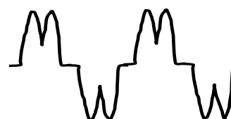
Typical current through LPF output stage
